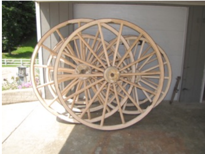
An impressive set of 6' chandelier wheels at Stutzman's Wheelwright's shop. Being produced for an interior fitting these wheels do not need to be made for strength and are therefore made from poplar.
