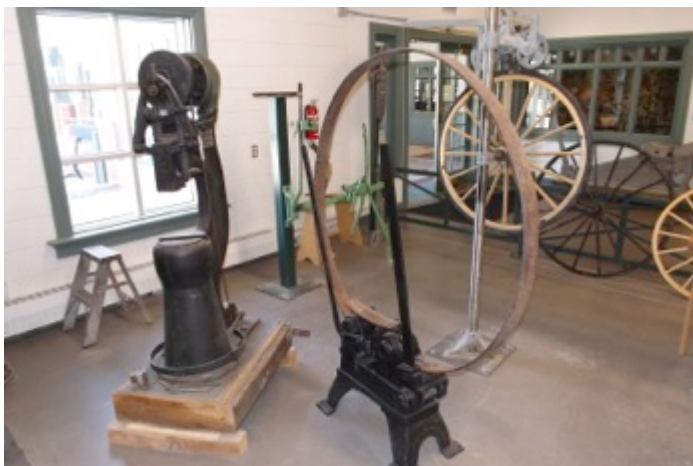
Original equipment in use at the Remington museum. Blacker power hammer (left), tyre setter (front right), rubber wiring machine (back right)
