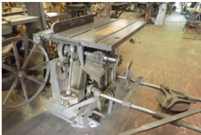
A view from Harley Chandler's Wheelwright's shop and a Variety woodworking machine from the 1800's specifically designed for wheelwrighting. Visible on this machine is a tonguing cutter for cutting round tenons on the outer end of spokes.
